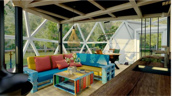
Wood platform diameter 12 m, House floor diameter 8 m, Center height: 4.0m, construction Aluminum frame, Roof: double layered laminated tempered glass (5mm tempered glass + 0.76PVB + 5mm, tempered glass) Window: 2 pcs, Entrance: 1 set of single glass door, Wind load: 150km/h, Snow load: 0.5kn/m2, 2000 liter water reservoir or permanet conect, biological sewage treatment plant, 6 KW solar electric system + wind turbin with batteries.
